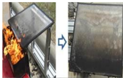
Fig. 11: Double glass after fire burning test
