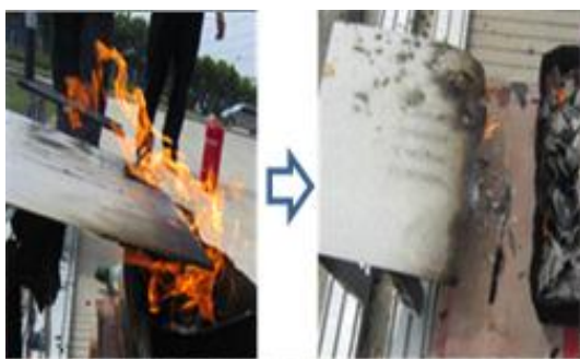
Fig. 10: Traditional module after fire burning test
