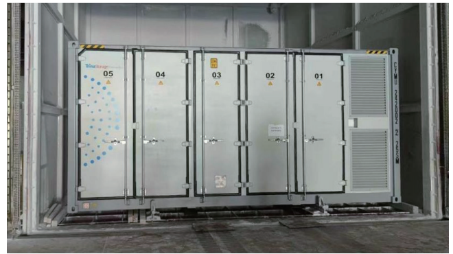
Figure 26 Battery compartment IP5X dust test
