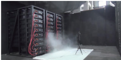
(c) Initiation of thermal runaway in Cell 37
