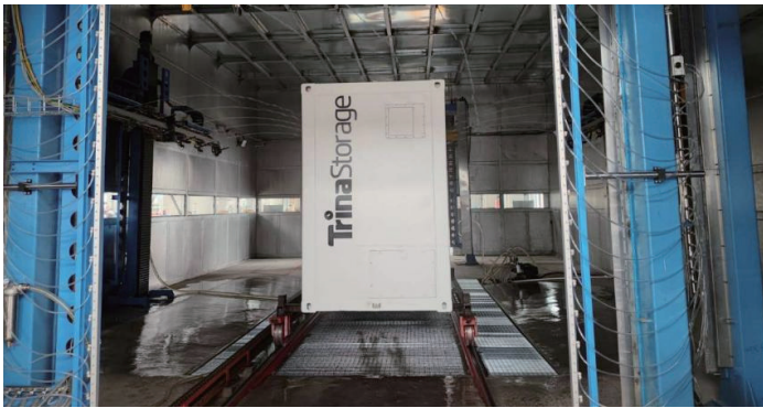
Figure 25 Battery compartment IPX5 waterproof product evaluation for IEC 60529 testing
