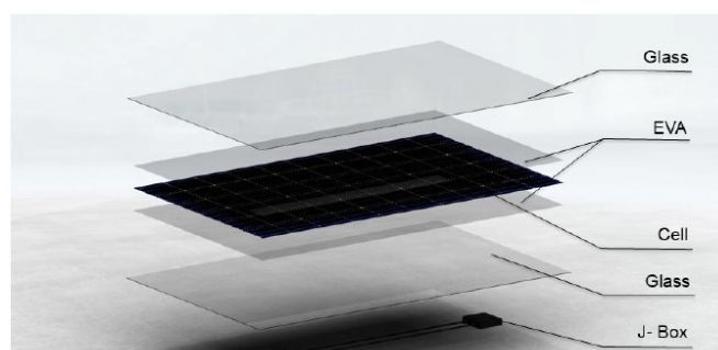
Figure 9. Dual glass module structure (layers)
