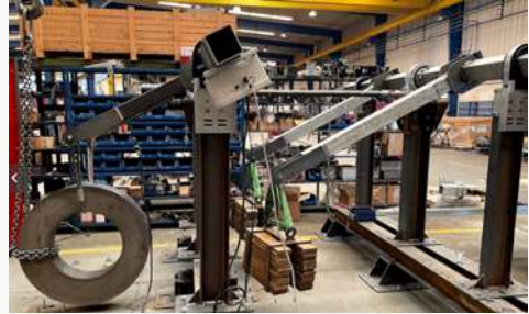
Image 17: Dynamic maximum load test
