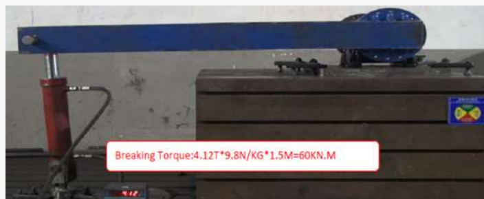
Image 16: Static maximum holding test
