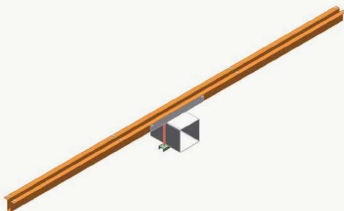
Image 8: Reinforced purlin design
