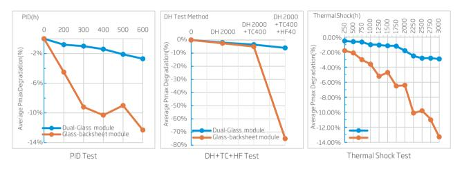
Figure 5. Pmax degradation of dual-glass module and backsheet module after long endurance test
