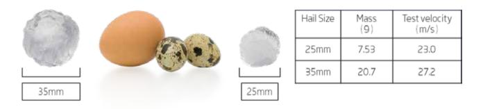
Figure 4. Comparison of hail size and test velocity
