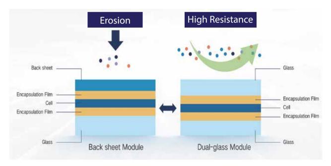
Figure 2. Comparing the structure of backsheet and dual-glass modules
