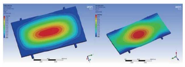
Figure 8. Deformation of backsheet (left) and dual-glass modules (right)
